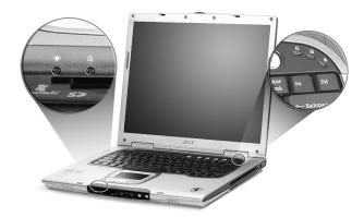
The Power and Battery status indicators are visible even when the display is closed.
